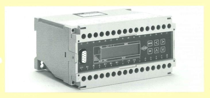
The microprocessor-controlled converter and switching instruments of the type series FT1400 are suitable for monitoring measured variables as a function of time, such as rotational speed, speed, clock rate etc. which can be converted to a proportional frequency by suitable speed sensors.
